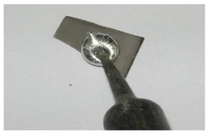
If you have a larger piece of InSn, place a small amount on an insulating material (here, a spare piece of a silicon substrate is used) and melt it using a soldering iron.
