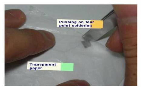
If to be used with the spring clip board, after soldering on the contacts, it is helpful to allow the contact to cool, and then using a plastic bag placed over the sample, use the flat edge of the razor blade knife to slightly mash down the contact so that it is flat on top. This will help the spring clip board pin make better contact.
