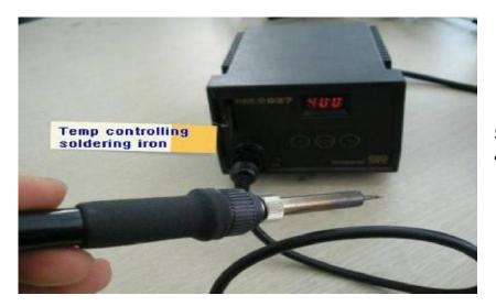
Set the soldering iron to 350°C to 400°C for best results.
