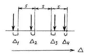
Probe displacements from equal distances.
