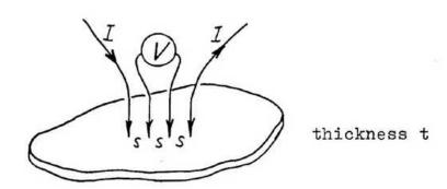
In the sections I. 1-4 and K. 1-2 we have given geometric factors for thin slices (t ≪ s) of finite extension. With the exception of section K.2, the resistivity was always written in the form:
