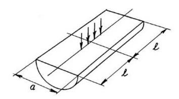
The geometric factor for an <u>infinitely long bar</u> of semicircular cross section is included in (d):
