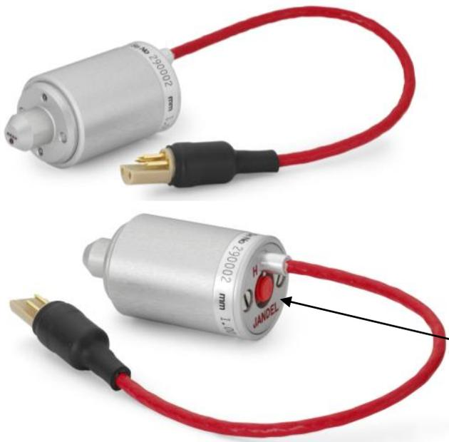
The Jandel Cylindrical four point probe has a user adjustable tip pressure that can be adjusted within one of three available pressure ranges by turning the small red knob on the top of the probe.
