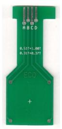
The HMS-3000 includes 5 of the SMB-20 sample mounting boards as shown to the left. This board requires manual installation of small wires. The SMB-20 can be used to mount samples up to 20mm on a side. You can read about the process involved in mounting a sample onto the SMB-20 sample mounting board here:
