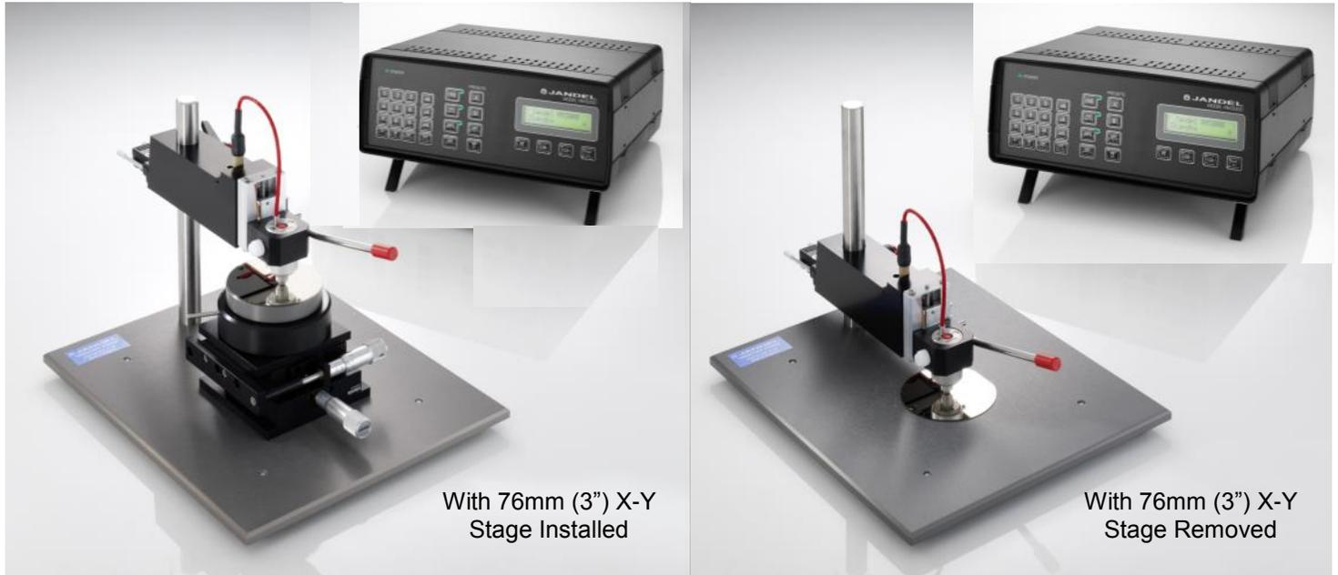
The **Multi Height Microposition Probe** combined with the **RM3000 Test Unit** is Jandel's most versatile four point probing system. It includes a fine X-Y stage for positioning small samples under the four point probe tips. The X-Y stage can be easily removed for measuring large samples such as substrates up to 10" x 10", or tall materials up to 6" tall.
